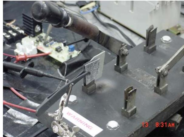
**PHOTO P1** 125 V Dc Knife Blade Apparatus - The knife blade draws the arc adjacent to the exposed material. Gaps are controlled to achieve arc voltages from 20 to 35 VDC
